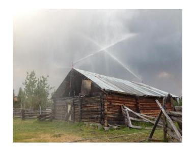
Since most homes and structures burn from windblown embers, keeping the roof and surrounding area wet can prevent the house from catching fire.
