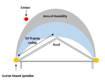
One kit will cover an average size North American home. If needed, additional mounts can be purchased individually. The sprinklers can operate at a very low pressure and are rated at 1.5 – 2.5 US Gallons. per minute.
